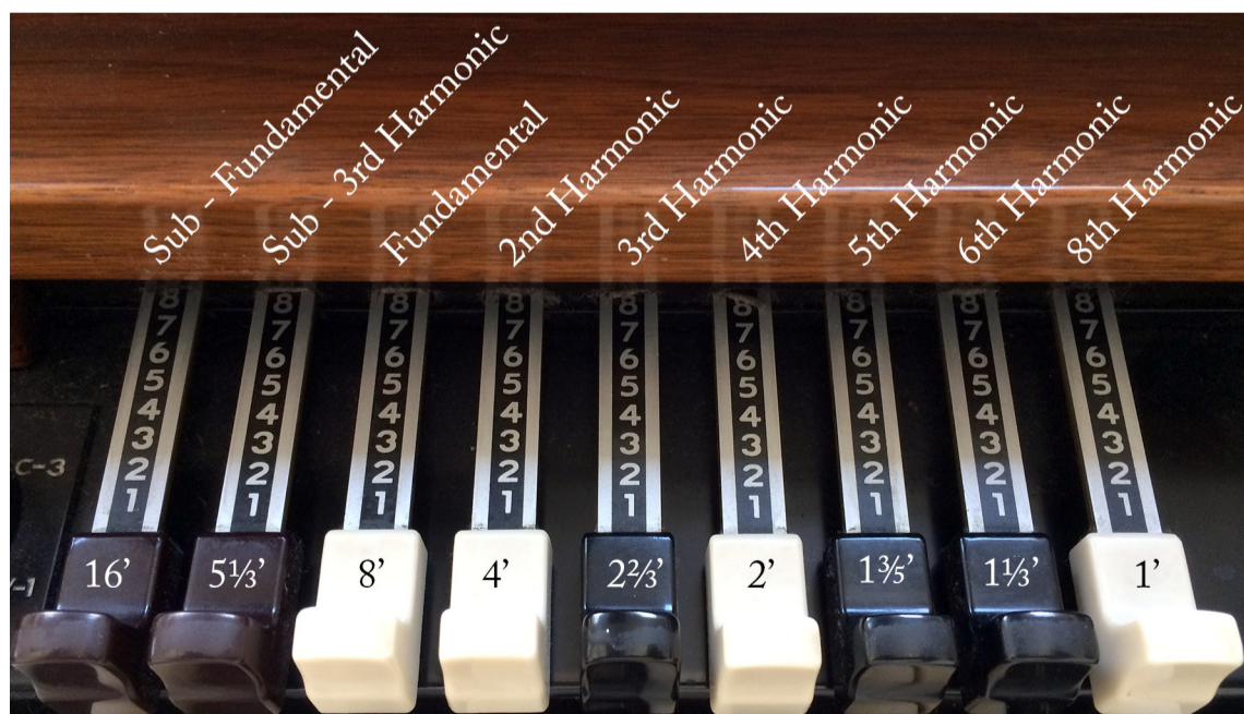
Figure 4.67 The 9 harmonic drawbars and their related pipe organ footages. This is the “all stops out” setting (888888888) and gives an aggressive, brass-like tone.
