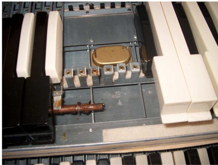
It may also happen that dendrites can be also found at the 'Preset Percussion Switch' located just underneath the 'B' preset key of the upper keyboard. Less usual than those found in upper keyboard.
