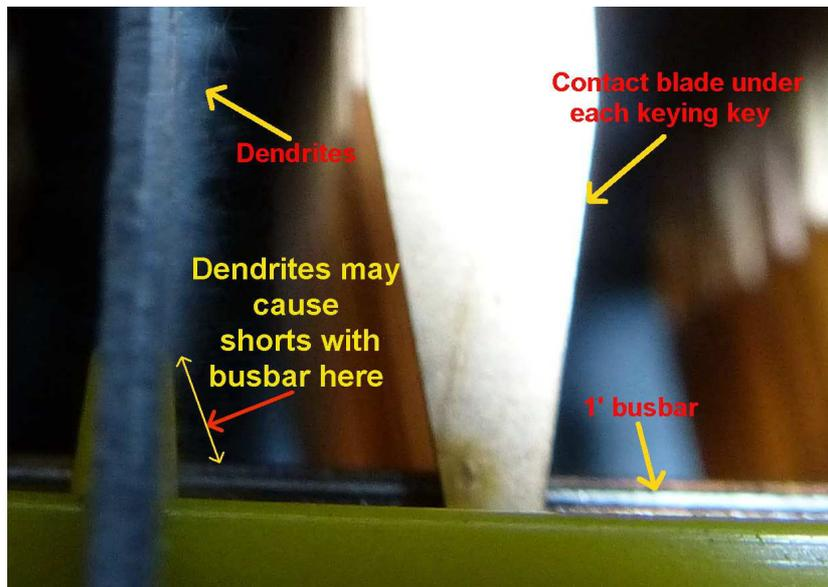
....bridging so permanently the 1' upper busbar to ground when "B" adjust key is pressed !
