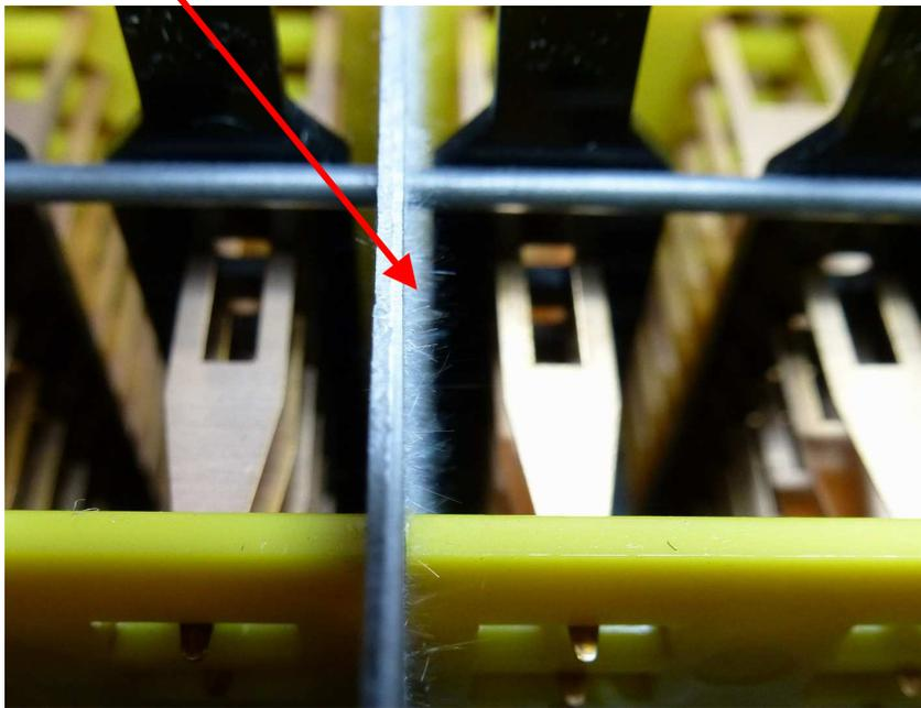
**After cleaning.** All dendrites particles removed on both sides.
