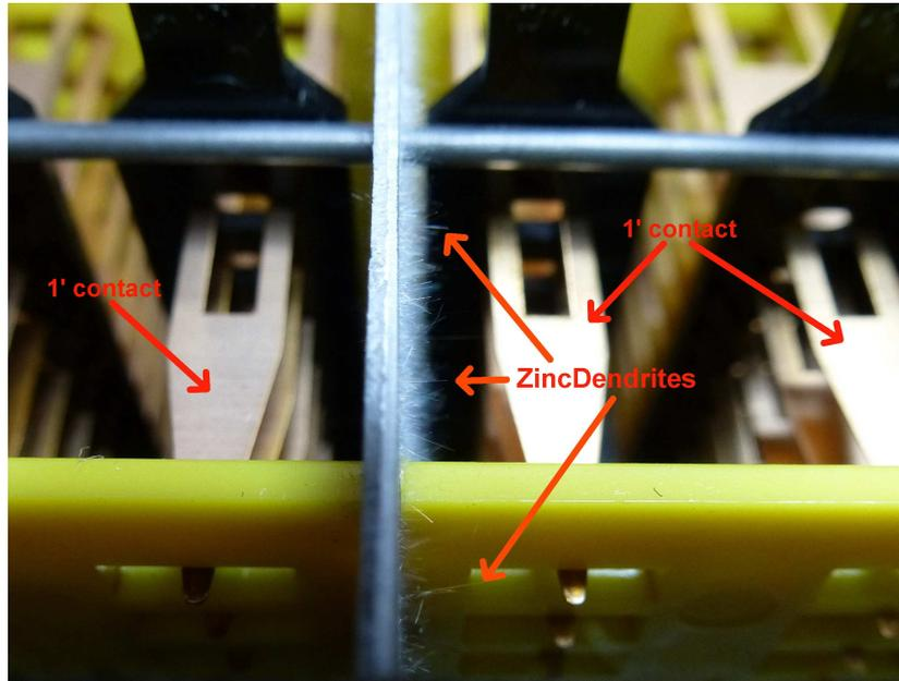
The little whiskers appearing on the zinc-plated metal plate when growing may touch the upper 1' contact blades and the 1' upper busbar....
